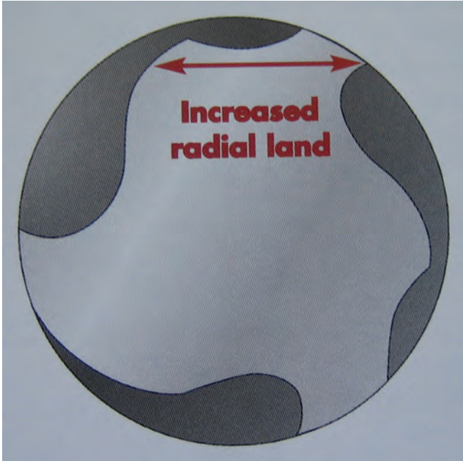
Figure 6-9. Cross-section of the K3 (SybronEndo) instruments that come only in nickel-titanium and as rotary instruments. The three blades are shaped much like a wood router, each blade with a sharp rake angle. The “tail” of two of the blades is ground short of the cavity wall, providing room for debris collection.
