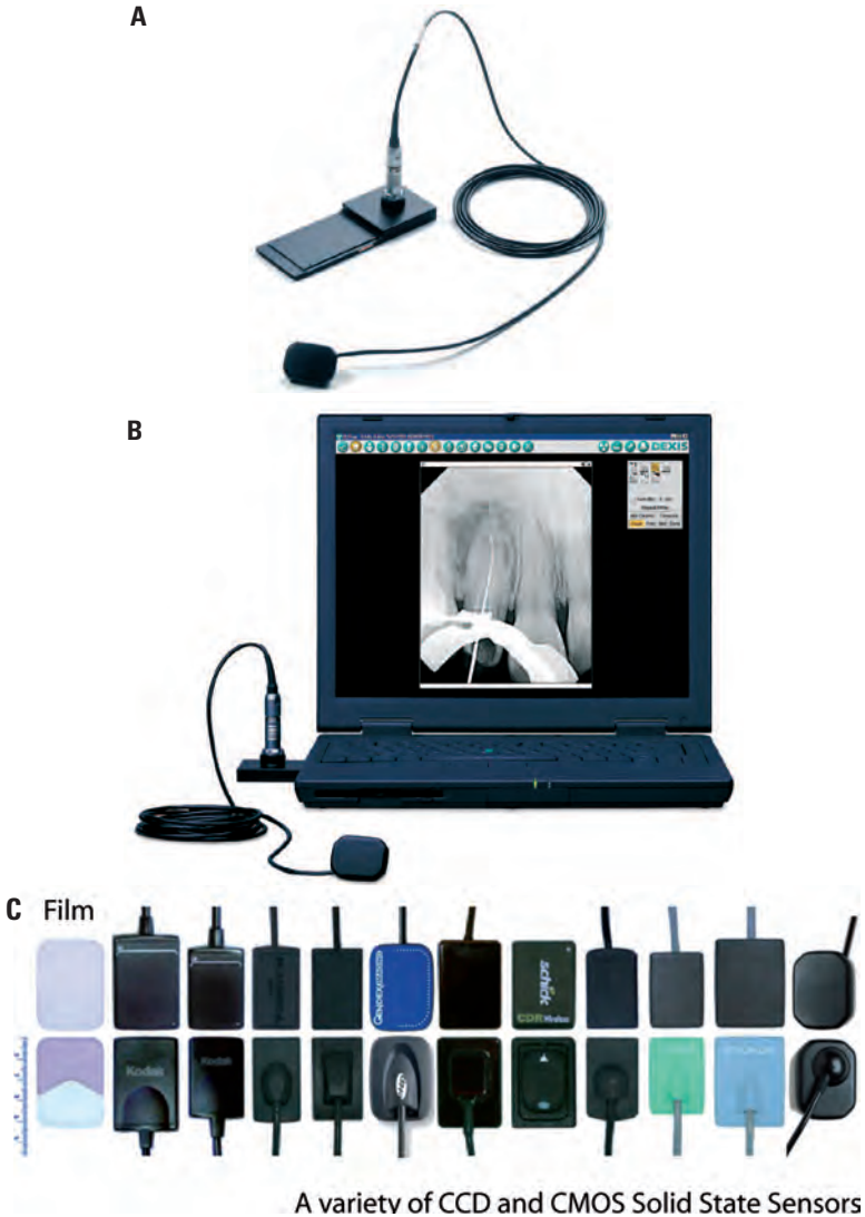
Figure 1-33. Completely portable direct digital radiography. A , PC Capture Card attached to an intraoral sensor. B , Capture card plugs into the USB port of the laptop computer, into which a software program has been installed from a CD-ROM. The image on the screen is the last scanned endodontic procedure. Total input is stored in the computer, where it may be modified, printed, retrieved at any time, enlarged on the screen and shown to the patient, and transmitted to the referring dentist or insurance company. C , Variety of CCD and CMOS Solid State Sensors.
