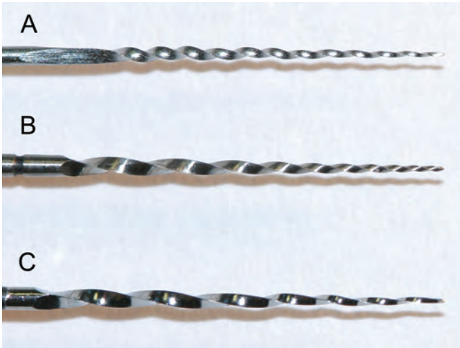
Figure 6-8. Comparison in pitch and helical angle in 3 comparable instruments: A , Sybron Twisted File (TF)—constant pitch and constant helical angle. B , Dentsply/Tulsa Profile Vortex—variable pitch and variable helical angle. C , Brassler-EndoSequence file—constant pitch and varied helical angle.
